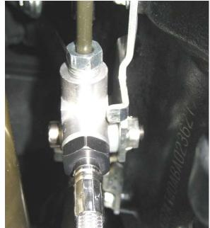
**Clutch hose (3):** Reroute the clutch hose behind the left slider-tube as shown in the picture.
