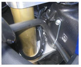
Make sure that no cable, hose or harness is bended and stays tension-free over the whole steering angle.
